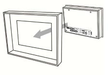
Step 3: Tighten the screws with the torque between 0.5 N-M and 0.7 N-M to avoid damage to the plastic case. DOP-110IG torque: 6.17 lb-inch (0.7 N-M)
