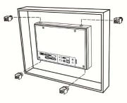
Step 4: For heat dissipation, please keep a minimum clearance of 60 mm (2.36 inches) and 45 mm (1.77 inches) respectively on the rear and bottom of the HMI.
